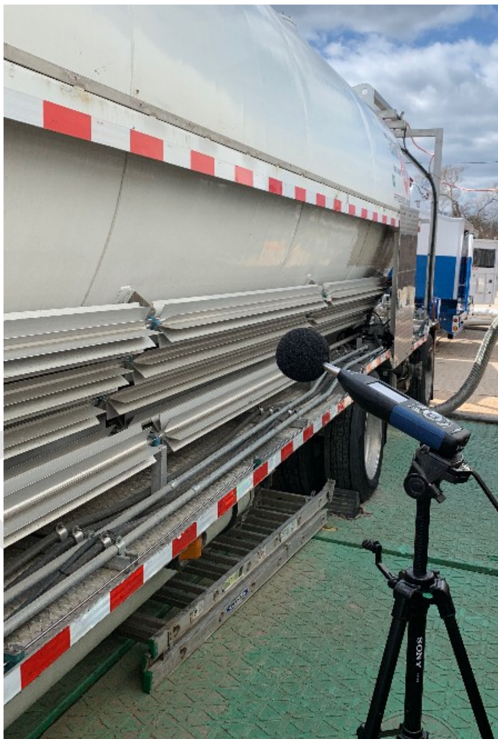
Figure 1. Noise Measurement Equipment recording noise from Site Machinery
