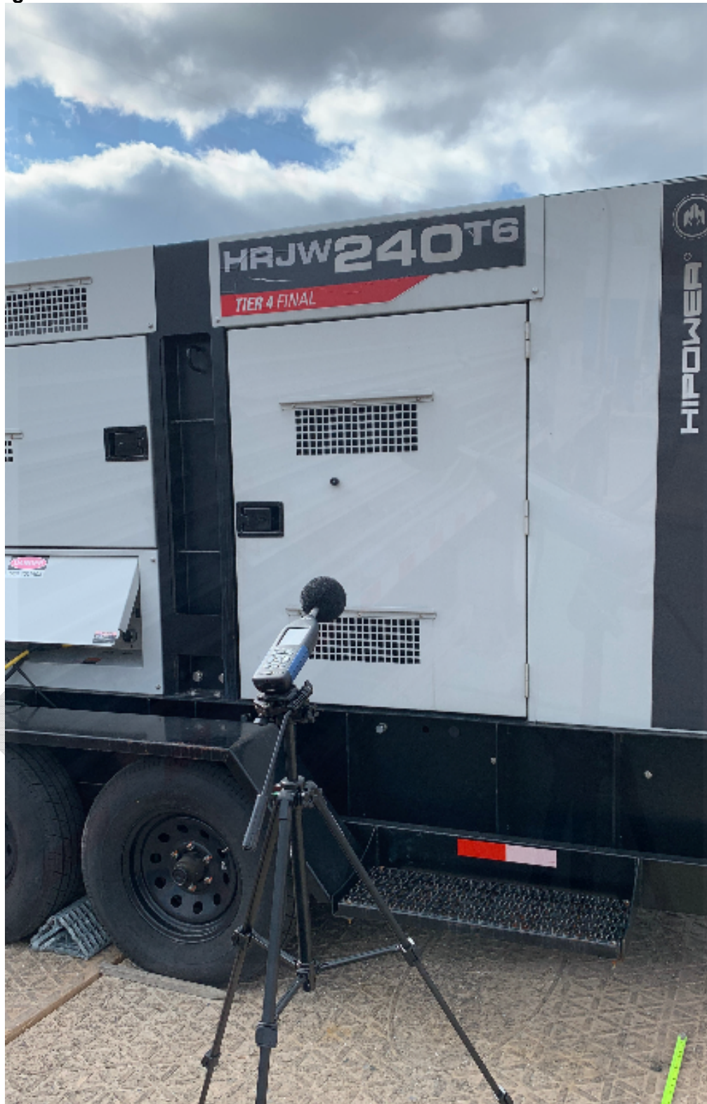
Figure 2. Measuring Noise from the Generator
