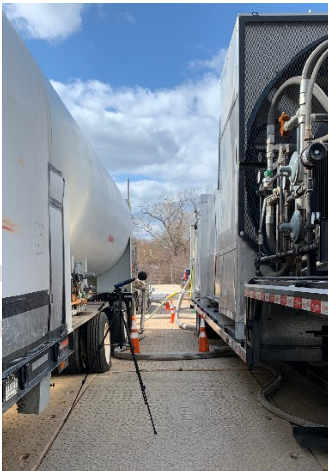
Figure 2. Noise Measurement Equipment recording Site Machinery
