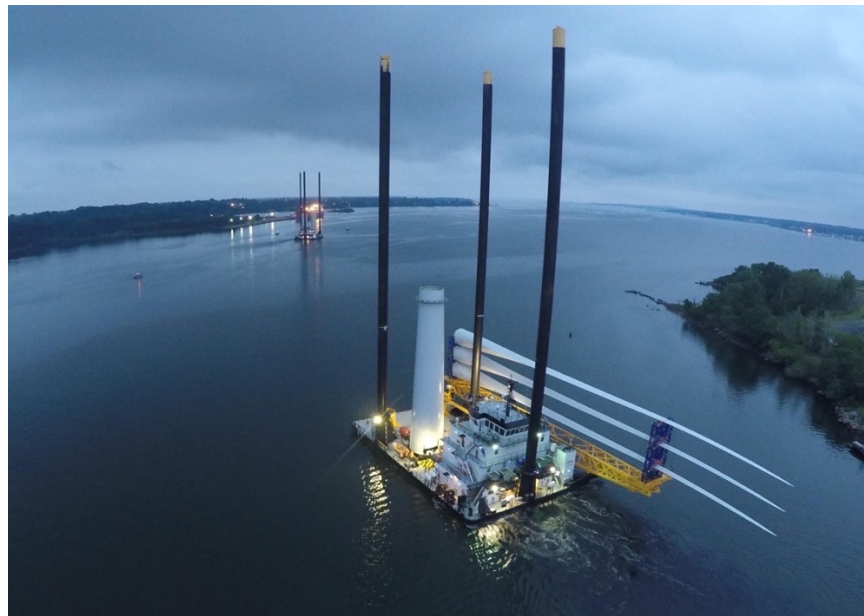
Figure 10-3: WTG transportation barges
