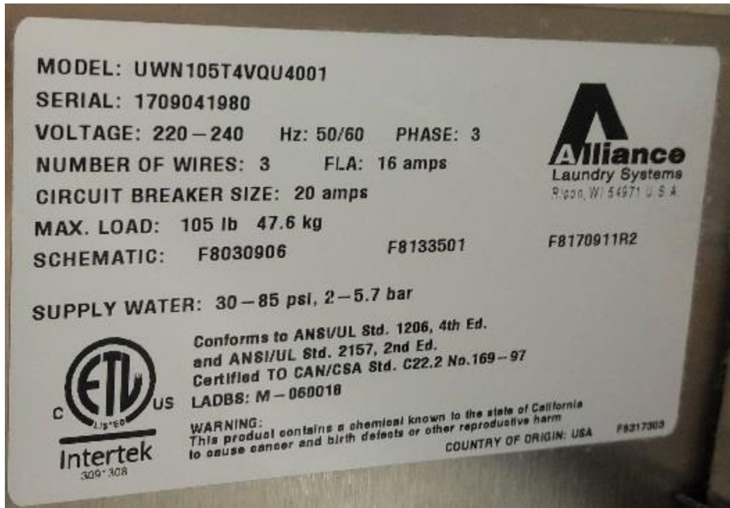
Figure 5-12. On-site Photo of Washer 2 Nameplate
