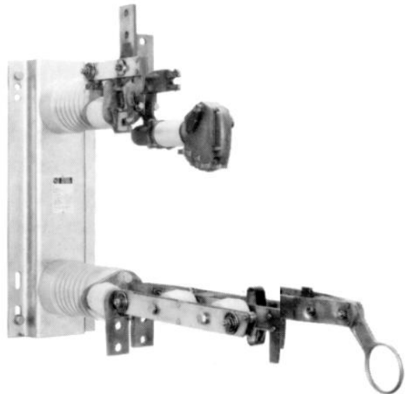
Figure 4 - Switch fully open. Voltage-regulator magnetizing-current interruption has taken place within the interrupter with no external arc or flame. Voltage regulator is de-energized and bypassed.
