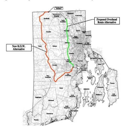
Figure 5.15: Proposed 115 kV line between Kent County and Sherman Road
