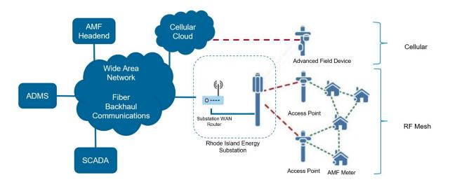
Figure C.1: Communication System with Fiber Backhaul
