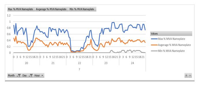
Figure 5.3.16: Example 5 Day Sample - Wind Generation Cycle
