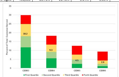
Figure 1.10 includes EEI survey information from utilities that benchmarked CEMI which is a reliability measure that tracks Customers Experiencing Multiple Interruptions, CEMI is a metric used to track pockets of customers whose reliability is poorer than average and may not improve while the overall system reliability is improving. Rhode Island Energy's CEMI performance is in the third quartile when compared to this EEI benchmarking.<sup>32</sup>
