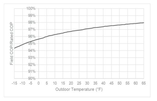
Figure 5.3.11: Impact of Temperature on Heat Pump Coefficient of Performance<sup>69</sup>
