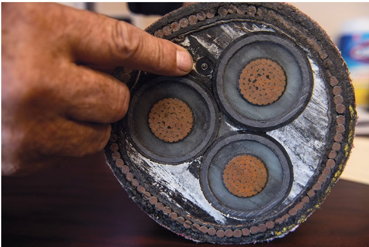
A section of the submarine power cable linking wind farm, island and mainland. Note the thin fiber optic cable, too. Neil Ever Osborne
