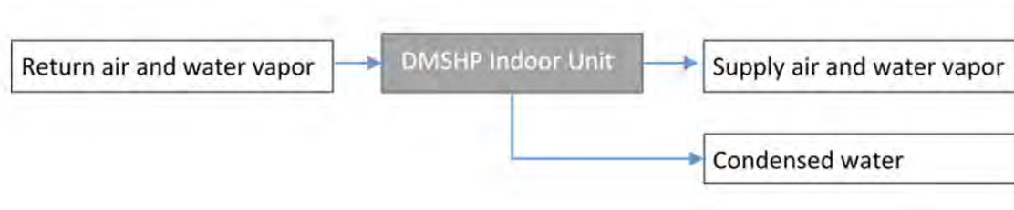
Figure 4. Indoor Unit Mass Flow
