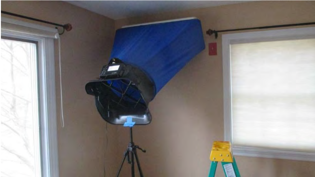
Figure 92. Non-Powered Flow Hood (Balometer) Setup
