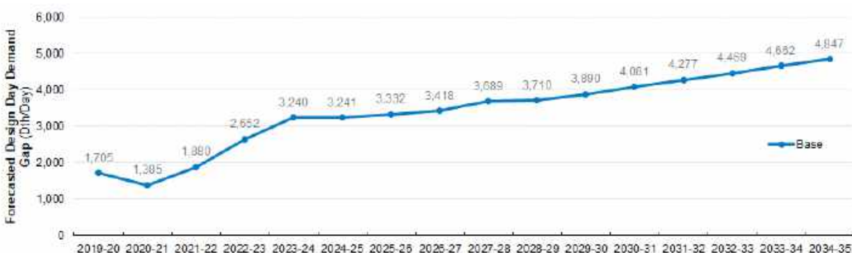
Figure 1: Capacity Constraint - Forecasted Gap Between Design Day Demand and Available Pipeline Gas Capacity for Aquidneck Island (Base Case Demand Forecast)
