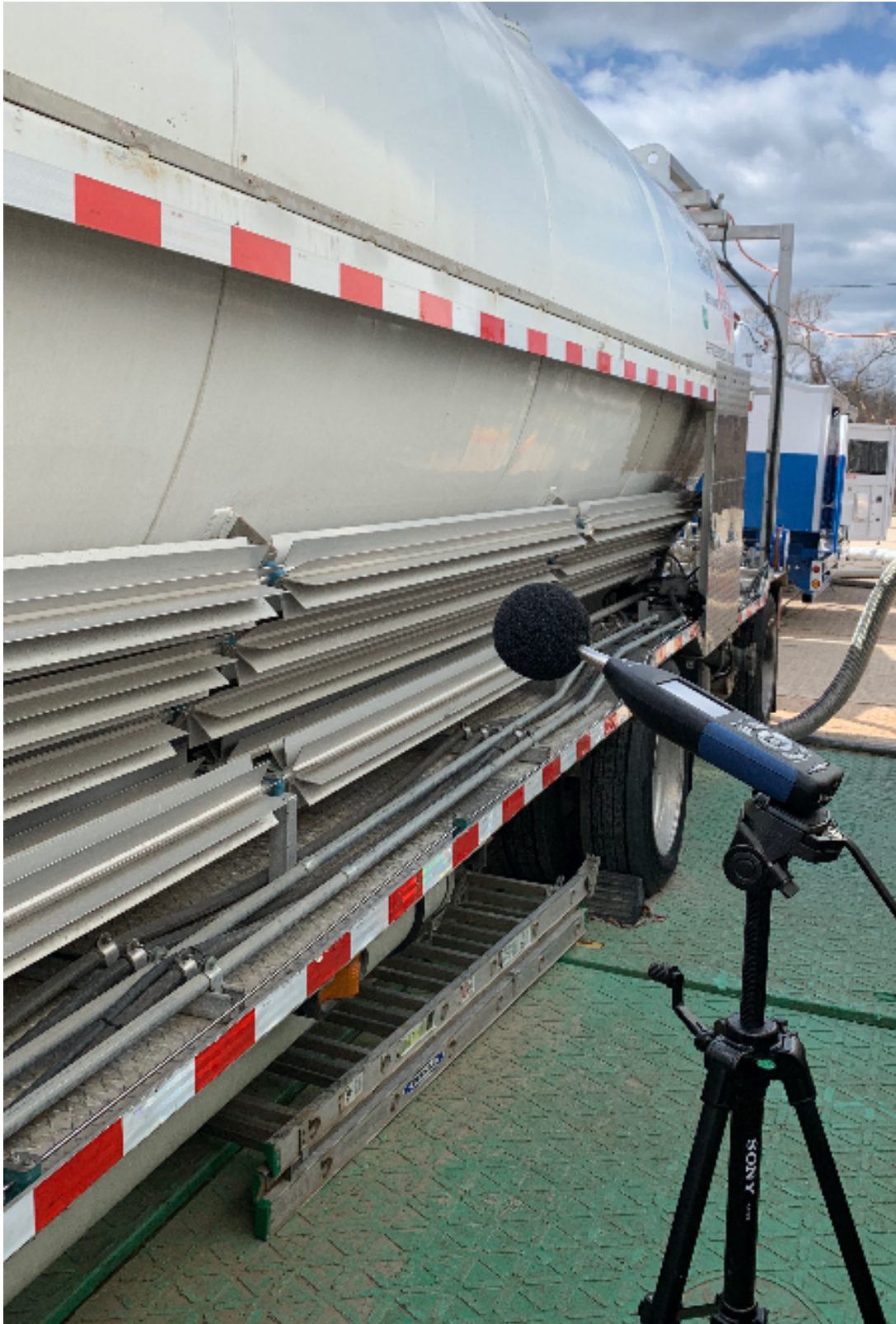
Figure 1. Equipment Noise Measurement
