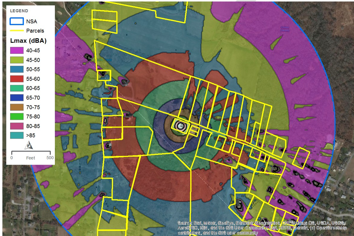
Figure 3. Modeled Lmax Noise Contours (Model 1)
