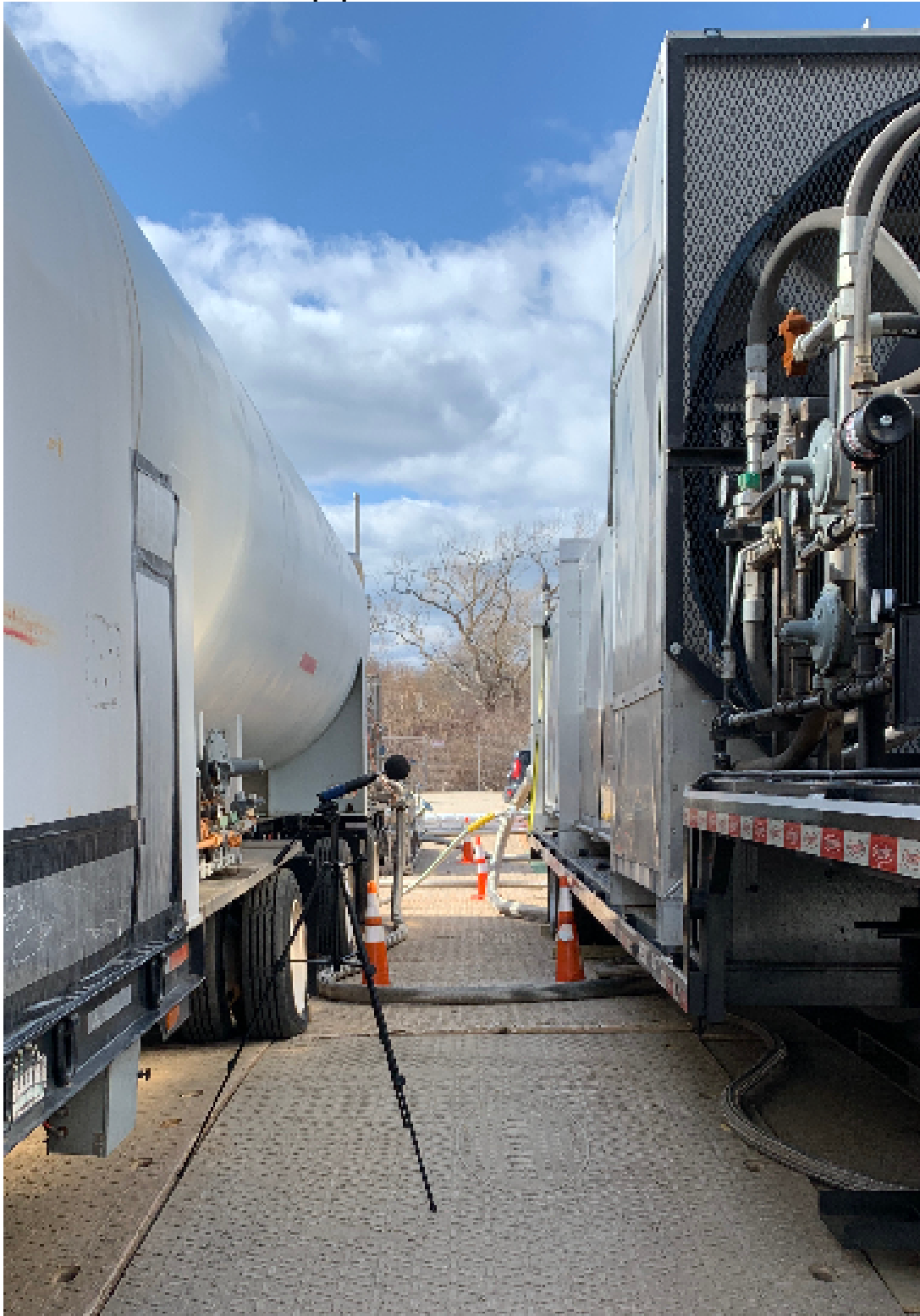
Figure 3. Noise Measurement Between Equipment
