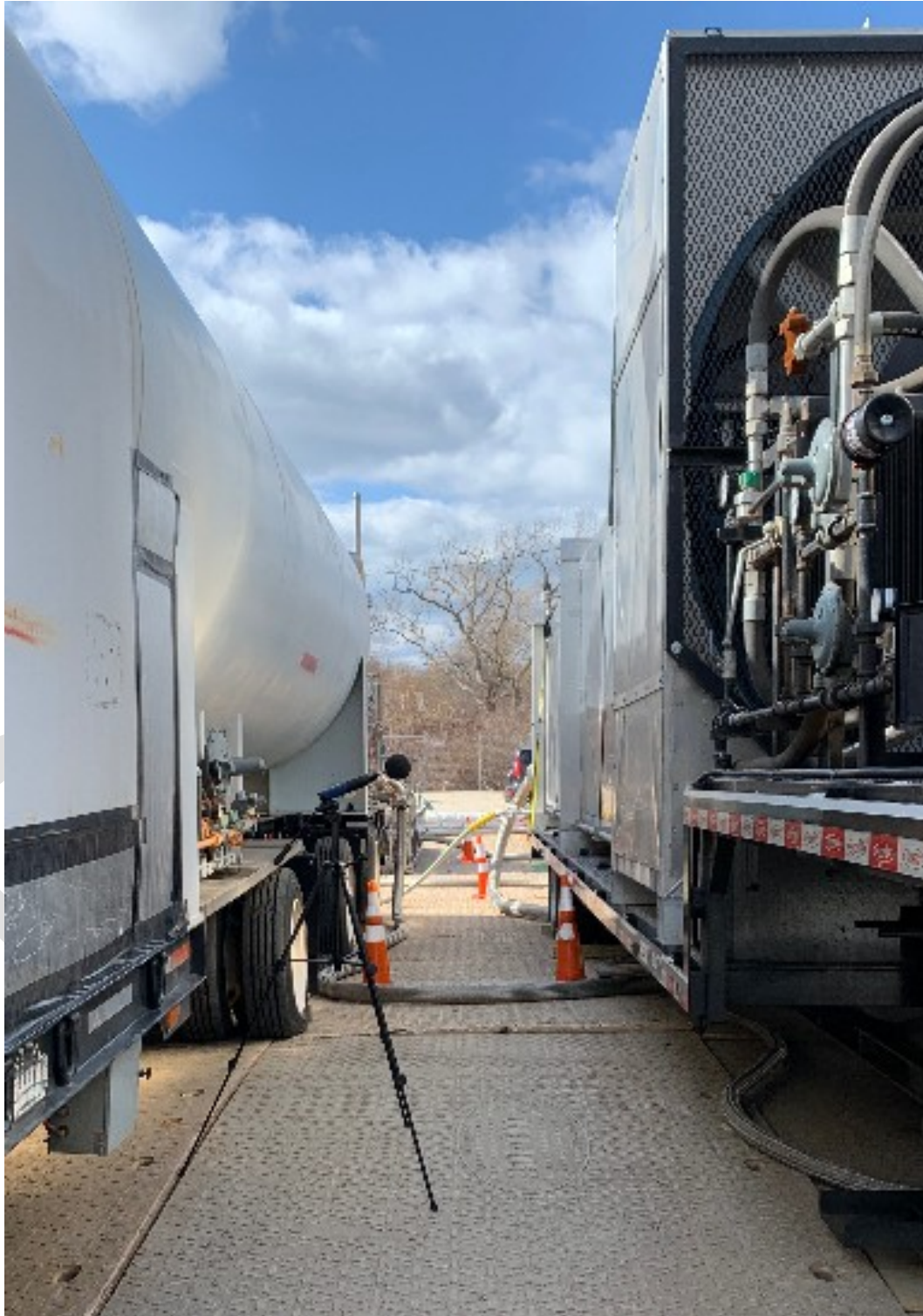
Figure 2. Noise Measurement Equipment recording Site Machinery
