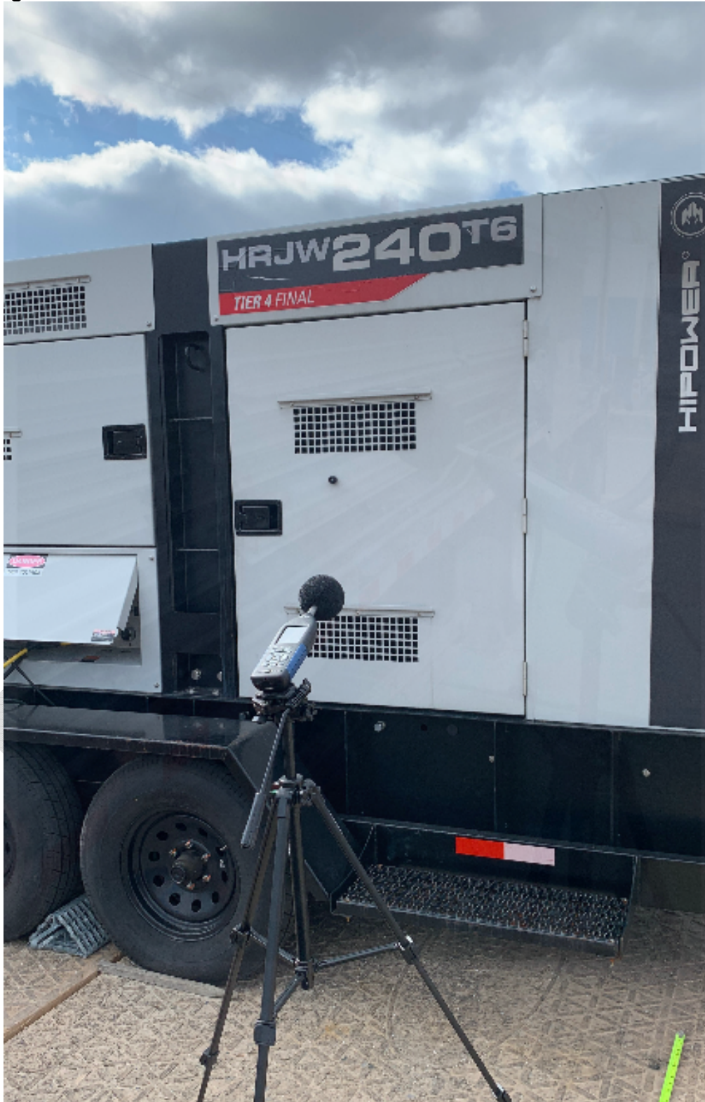
Figure 2. Measuring Noise from the Generator
