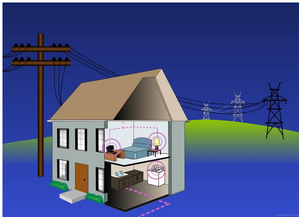
Figure 1. Numerous sources of ELF EMF in our homes (appliances, wiring, currents running on water pipes, and nearby distribution and transmission lines).
