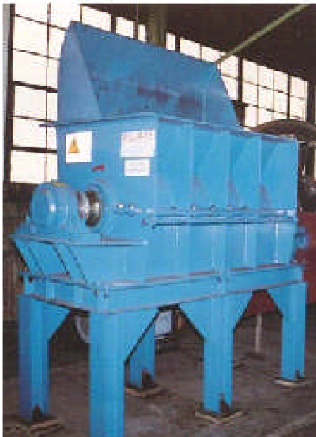
Figure 7: Typical Hog (Chip Grinding Device)
