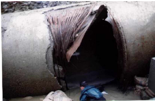
Rupture of the 102" Aqueduct – November 17, 1996
