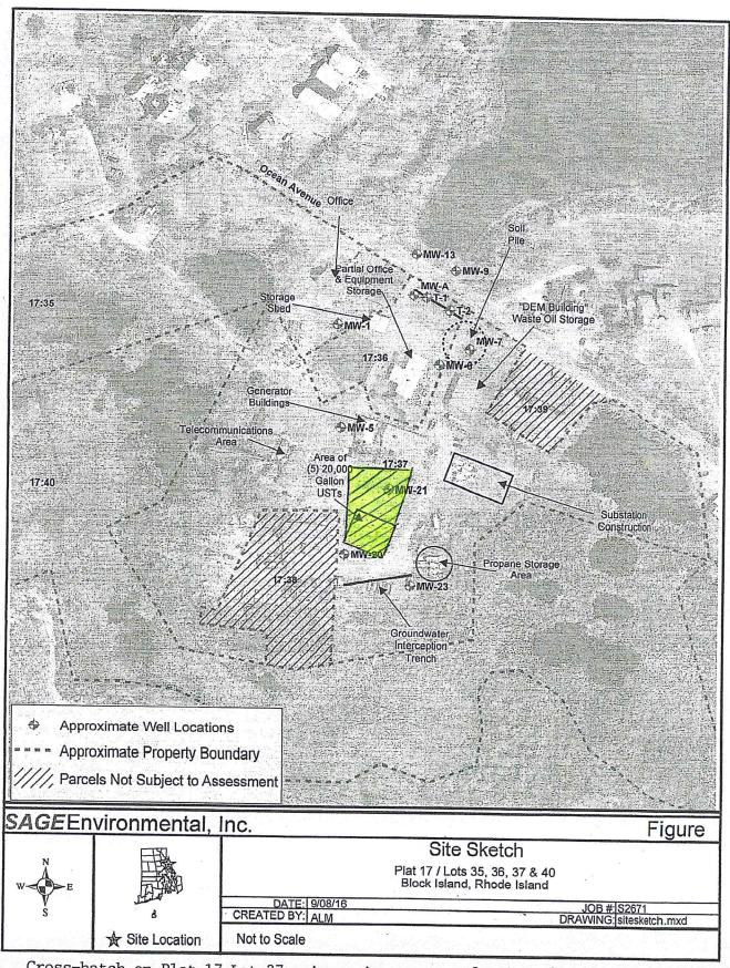
Cross-hatch on Plat 17 Lot 37 = Approximate area of original tank farm. MW-20 = Area of 5 remaining tanks from the tank farm to be removed. MW-21 = Approximate area where new replacement tanks will be located.
