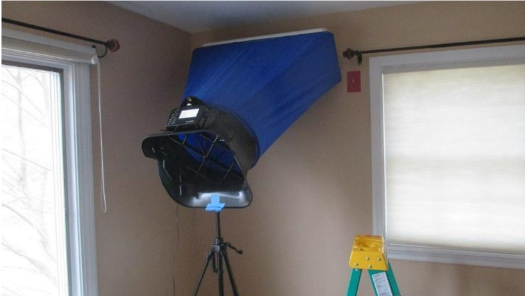
Figure 92. Non-Powered Flow Hood (Balometer) Setup
