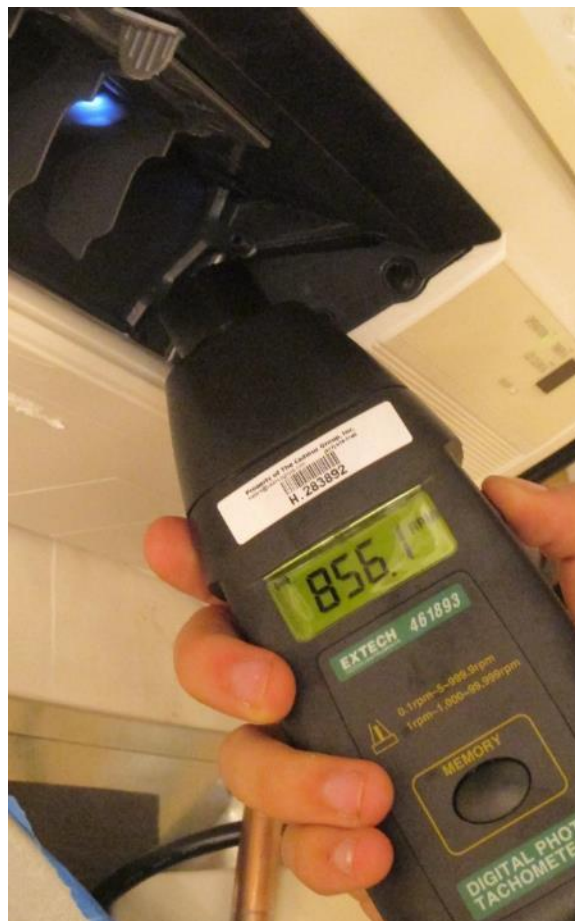
Figure 85. Optical Tachometer Data Collection
