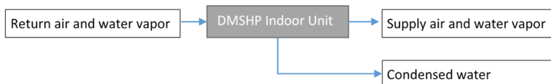
Figure 4. Indoor Unit Mass Flow
