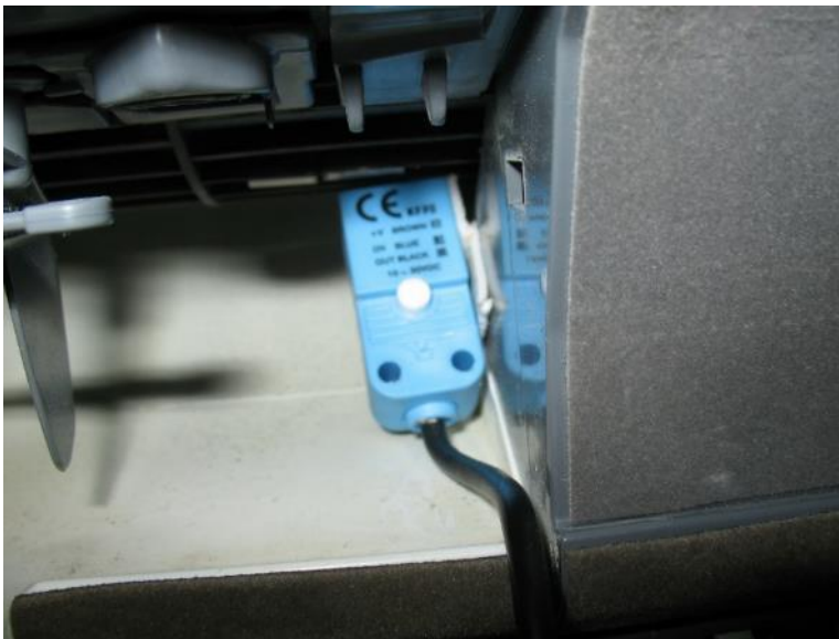
Figure 84. Proximity Sensor Arrangement (NREL Image 18330)
