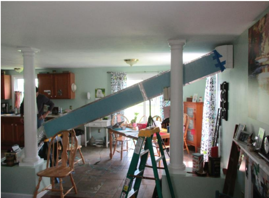
Figure 90. Extended Testing Site B: Large-Unit Powered Flow Hood
