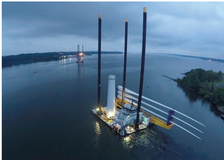
Figure 10-3: WTG transportation barges
