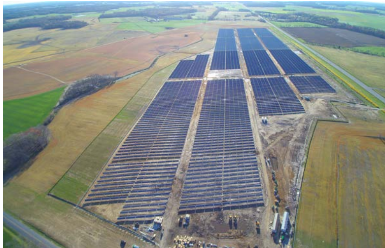
Figure 2: The 13 MW system installed for Johns Hopkins is expected to offset about 18% of the total campus energy usage.
